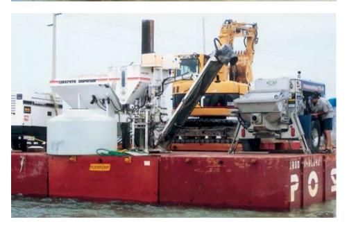
The barge used every inch of space to hold a variety of equipment – a trailer pump, batch plant, air compressor, welder, excavator – along with several gallons of fresh water and numerous thousand pound bags of cement, sand and other ingredients needed to produce concrete on board.
